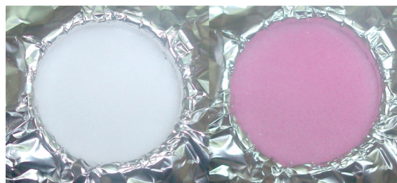
Figure 1. Photographs of silica gel doped with compound 3a , in an aluminum sheet, before and after UV irradiation (365 nm) for 15 s.
